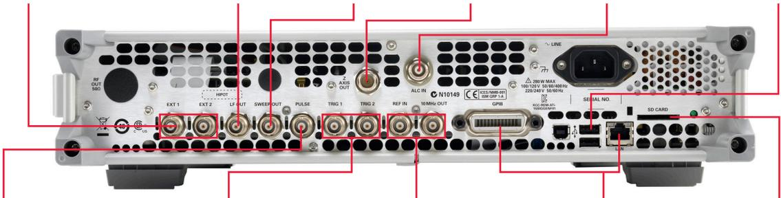
Supply input-pulsed TTL or CMOS signals < 20 ns for pulse modulation.
